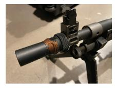
it is recommended to evenly apply a high-temp copper antiseize to external threads and the gas seal taper of the muzzle device. Ensure device is clean and free of oil and debris.
