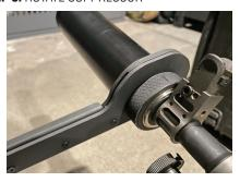
Close retaining jaw on tool if not already. Rotate the suppressor clockwise (from the muzzle) or in the direction of the UNLOCK arrow.
