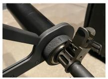
Utilize the locking wrench over the wrench flats to engage the suppressor. This will ensure positive retention when hot and aid in breaking any "locking" experienced from excessive use.
