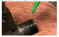
With a standard solvent, such as acetone or MEK, clean the barrel threads using a brush and rag. allow solvent to dry and repeat process as necessary until any oil is removed.
