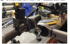
It is recommended to apply a small amount of thread locker such as Rocksett to the barrel threads. This will aid in ensuring the muzzle device will remain in place under extreme duty.
