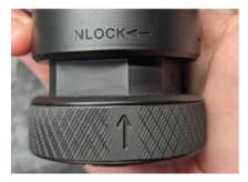
Rotate the locking collar to the UNLOCK position as indicated by the arrow direction and its final position pointed at the tip of the suppressor body arrow.
