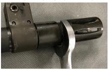
Utilizing available wrench for servicing weapon, remove existing muzzle device.
