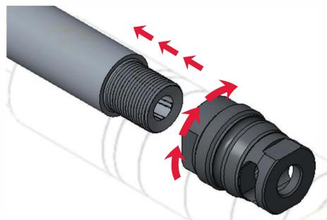
**Note:** If the Regulator mount loosens due to extreme heat cycles, then it's recommended to degrease the threads and use a high temperature threadlocker. LMT AT recommends using a medium strength, high temperature threadlocker like Hot Lock or Rocksett.
